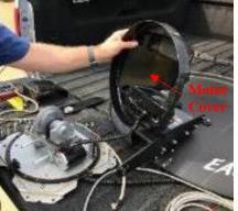
5. For existing two-piece split Motor covers: Remove the 7 bolts from the split cover and remove the cover.
