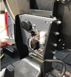
3. Now move to the other arm bracket (cable harness side) and remove all 8 bolts like the previous side, starting with the 4 bolts at the bottom of the arm. You will need to hold the antenna reflector with your left hand to balance the dish.
