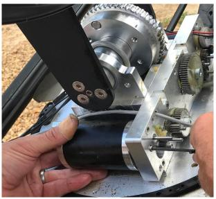
Note: When reassembling the Motor Cover make sure the Cable Harness rubber plug is securely seated.
