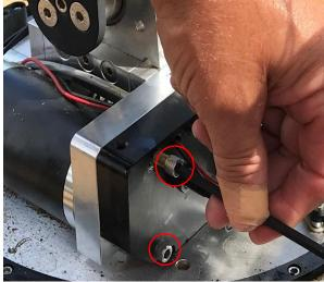
9. Remove the **4** screws holding the Motor onto the Gear Box. Sometimes, because of the grease, the gears come out with the gray cover when you open the gear box. This is normal.
