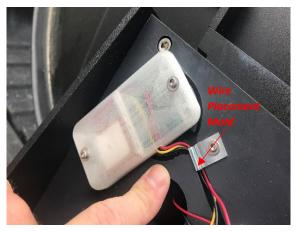
9) Reattach the wires in the correct placement (2 red wires together, 1 yellow wire and 2 black wires together) plug your controller back in and run a test.
