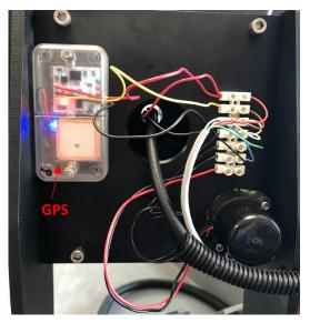
Using a jewelry screwdriver, unscrew the top three left hand side wire holes.
