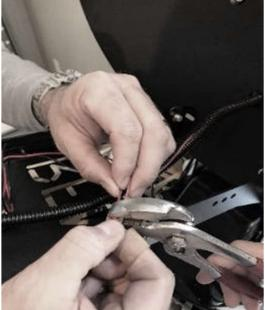
11. Route the Cable Loom down either side of the LNB Arm and secure with Cable Ties (provided).
