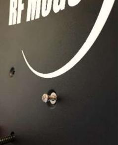
9. Attach the LNB Arm (choose your direction on Page 13 based on your provider) loosely to the Reflector using 4 of the  $\frac{1}{2}$  - 20 x  $\frac{3}{4}$  screws provided. The LNB Arm should be able to be pivoted upwards into the Reflector after it is attached. Tighten all 6 screws using a #3 Philips screwdriver.
