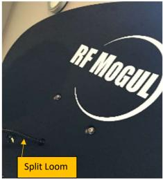
8. Attach the Reflector loosely to the Brackets on the Mount in the top 2 holes using 2 of the  $\frac{3}{4}$ "-20 x  $\frac{3}{4}$ " Philips SS screws that are provided. Align the remaining 4 holes then tighten the top 2.
