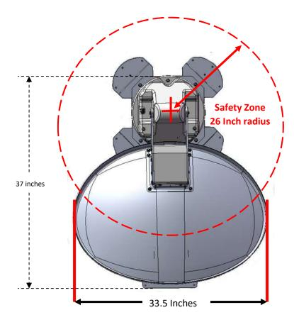
Rotational clearance from center rotation point is 26 inches when dish is elevated and rotating. This is a safety zone. Anything higher than 6 inches within this zone is at risk.
