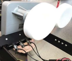
17. **Attach** the two (2) LNB Arm Stow Brackets on the <u>inside</u> of the LNB arm assembly (<u>see diagram</u> <u>below to determine direction</u> arm brackets and LNB should be placed) using the screws provided and then **secure** both the *two inner* and *outer screws* that hold the LNB into place.
