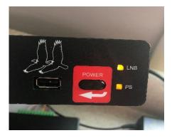
14. (If you are receiving a <u>new</u> controller, the software is already preloaded, so you will not receive a USB jump drive for it. Go to the next step) Power the RF Mogul antenna controller back **ON** and insert the USB JUMP Drive that has the RF Mogul antenna controller software loaded on it. The LCD display should change and show that the software is downloading. When the software download is complete, remove the USB JUMP drive.
