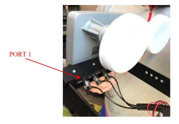
9. **Splice** the Black and Red wires using the Scotch-Lok connectors (red button). It is not necessary to strip the wires. Place the ends of the wires deeply into the connector and pinch with pliers. This will connect the LED's that will reflect onto the dish at night. Tuck the Scotch-Lok connectors through the hole in the dish.
