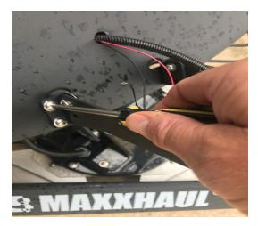
7. **Attach** the new LNB Arm loosely to the Reflector using 4 of the ½ x 20 x ½ inch screws provided. The LNB Arm should be able to pivot upwards into the Reflector after it is installed. Tighten all four (4) screws down tight at this point.
