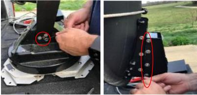
2. After removing the arm bracket, you will expose the elevation shaft cap. *Note-Elevation Shaft cap comes off groove side inward!*
