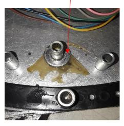
10. Place the Flipper on top of the washer.
